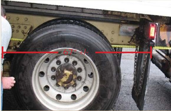
67" from the center of the tandem to the body hinge pin (see photo above) allows the frame to extend into the paver. If the afterframe dimension is correct, there should be 46" from the center of the rear axle to the end of the body as well as approximately 75" from the center of the tandem axle to the end of the frame.
